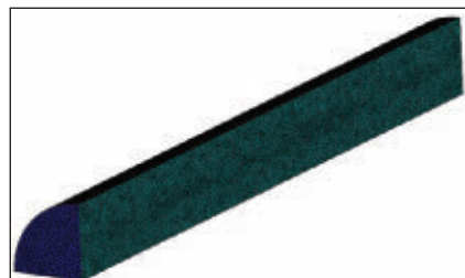
▲ Fig. 2 Analyst and analytic transmission phase agree to four decimal places of accuracy for this circular waveguide.
